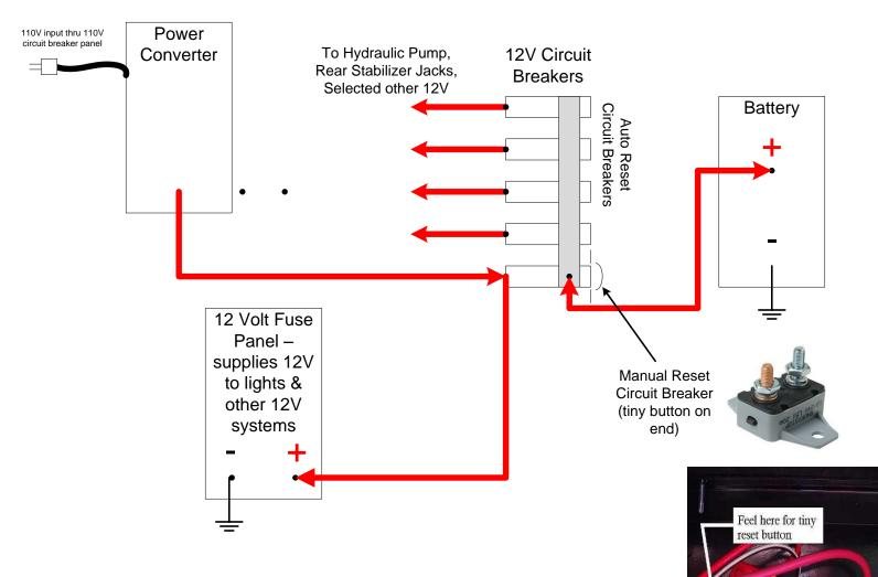
When plugged into shore power, 110V is supplied to the main circuit breaker panel inside the RV. One of those circuit breakers supplies power to an outlet, usually found behind the basement wall, into which the Power Converter is plugged.
